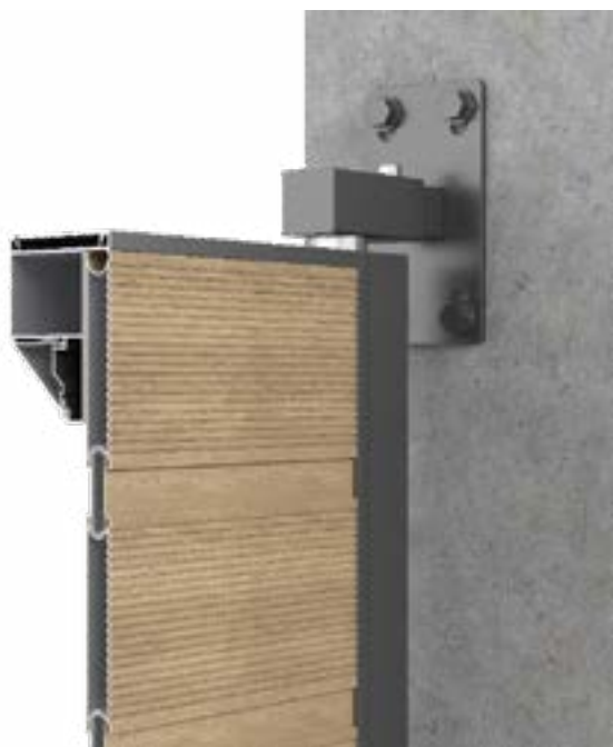
Detailed views of the sash and grooved profiles, along with the pivot axis profile with INOX 316 PIN able to hold 250 kg each. Maximum single door sash is close to 4m 2 withstanding a maximum wind load of 2KPa.
